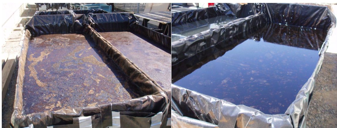
Fig. 10. Immediately after applying crude oil to the water (10/2/07), treated with SphagSorb (left) and untreated (right).
