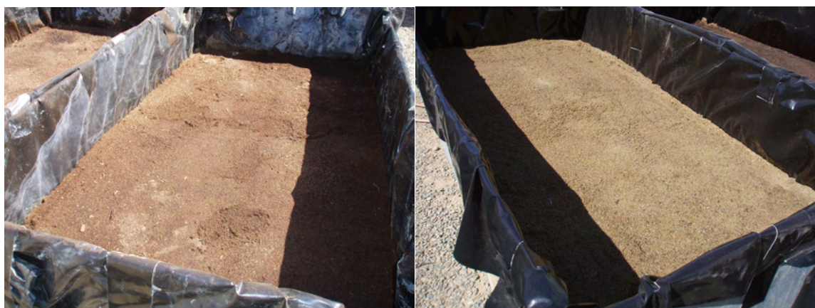
Fig. 9. Immediately after applying diesel oil to the sand (10/2/07), treated with SphagSorb (left) and untreated (right).
