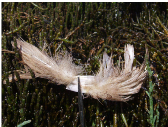
Fig. 17. Feather after wiping crude oil on pickle weed, one week (10/8/07) after application, treated with SphagSorb (left) and untreated (right).
