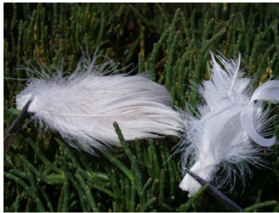
Fig. 18. Feather after wiping diesel oil on pickle weed, one week (10/8/07) after application, treated with SphagSorb (left) and untreated (right).
