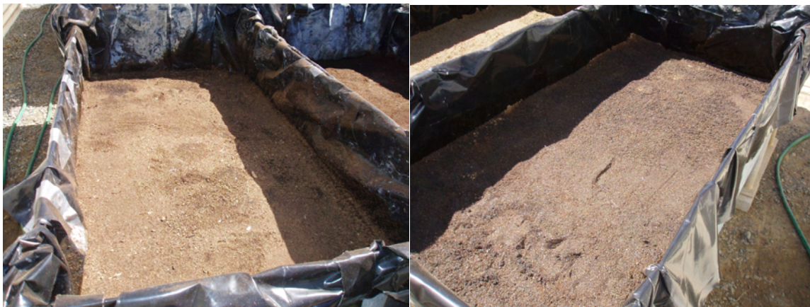
Fig. 8. Immediately after applying crude oil to the sand (10/2/07), treated with SphagSorb (left) and untreated (right).
