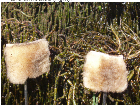
Fig. 19. Fur pad after wiping crude oil on pickle weed one week (10/8/07) after application, treated with SphagSorb (left) and untreated (right).
