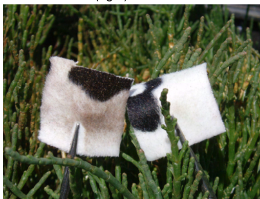
Fig. 22. Polypropylene cloth after wiping diesel oil on pickle weed one week (10/8/07) after application, treated with SphagSorb (left) and untreated (right).
