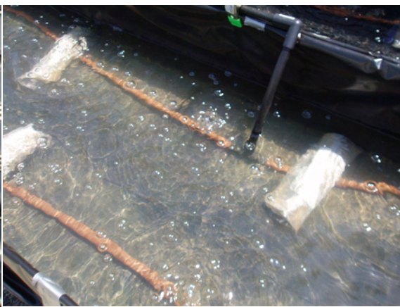
Fig. 2. Close-up of aerators and sand bags before adding Perlite growth medium.
