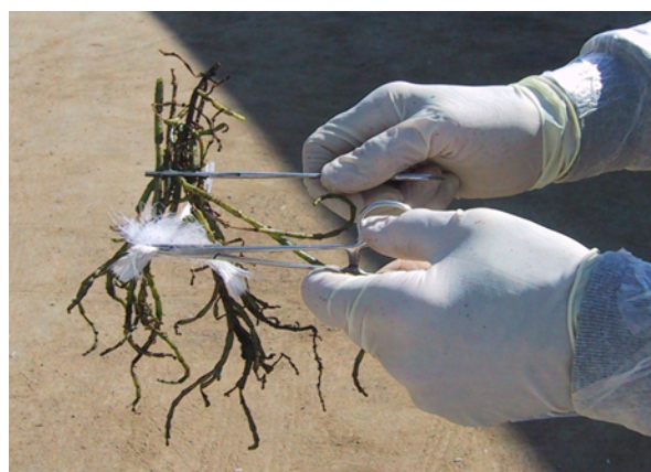
Fig. 16. Wiping technique for testing the oil stickiness, shown with crude oil on pickleweed.
