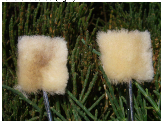
Fig. 20. Fur pad after wiping diesel oil on pickle weed one week (10/8/07) after application, treated with SphagSorb (left) and untreated (right).
