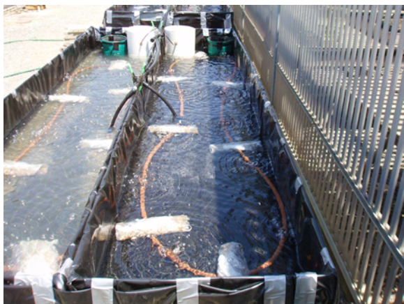
Fig. 1. Plant tanks with aerator tube held in-place with plastic bags of sand before adding Perlite.
