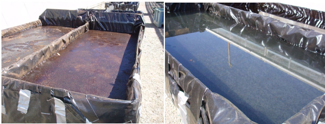
Fig. 11. Immediately after applying diesel oil to the water (10/2/07), treated with SphagSorb (left) and untreated (right).
