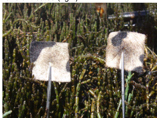
Fig. 21. Polypropylene cloth after wiping crude oil on pickle weed one week (10/8/07) after application, treated with SphagSorb (left) and untreated (right).
